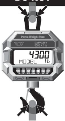
**DO NOT INTERFACE HARDWARE (SHACKLES, HOOKS ETC.) THAT ARE OVERSIZED AND RESTRICT SINGLE POINT LOADING AND SELF-ALIGNMENT WHICH CAN RESULT IN OFF-AXIS LOADING.**
