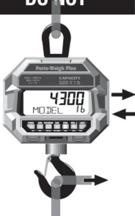
**1. DO NOT PUSH OR PULL ON A LOADED SCALE.
