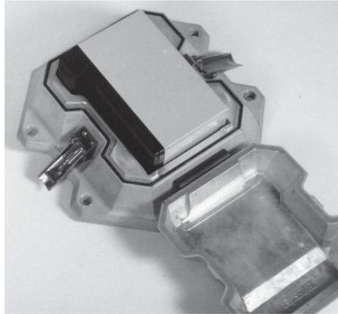
The Port-A-Weigh is powered by a 12 volt rechargeable battery. The battery is located in the rear compartment of the scale. Two stainless steel fasteners secure the battery access door. To remove the battery for charging; unlatch the fasteners and pull the battery straight out. The battery will automatically disengage from its connectors and may be plugged into the battery charger for recharging.
