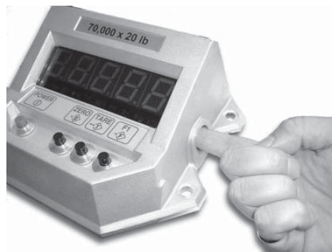
(Left) Seal Port removed and CAL Switch Button shown (Right) Pressing CAL Switch Button with tip of finger
