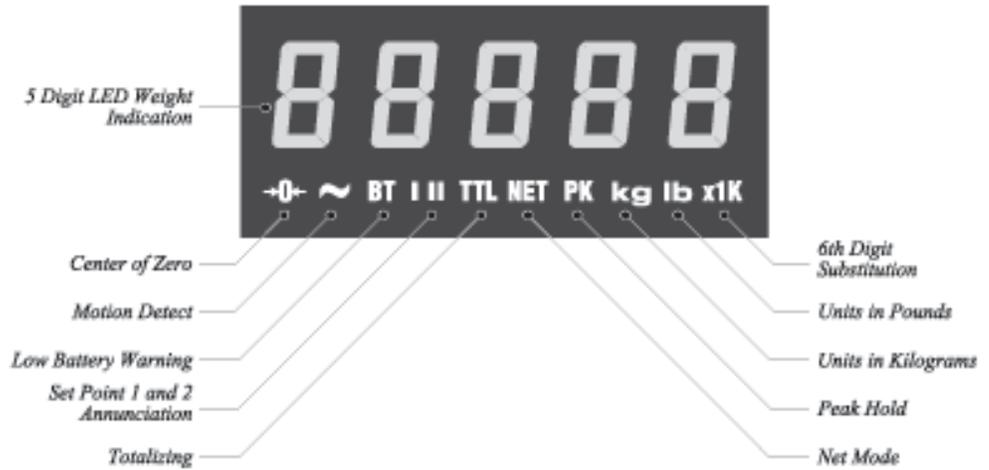
*In the event of an overload condition, the display will flash a warning to the operator.*
