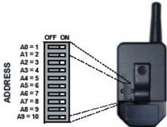
MSI supplies the transmitter and receiver as a matched set with the DIP switches already configured. A replacement RFRC will only need to have the transmitter DIP switches set. To change the DIP switch in the receiver requires disassembly of the crane scale front casting.
